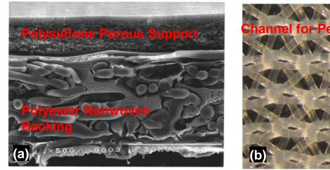
**Figure 3.** (a) Magnified cross-section of a typical composite polyamide membrane and (b) a top view of a permeate spacer showing channels for water flow.
