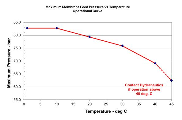
**Figure 4b.** Temperature versus Pressure Operation Limits for Seawater Membranes\*-Metric Values:
