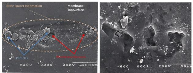
Figure 2. Membrane surface abraded by particles.
